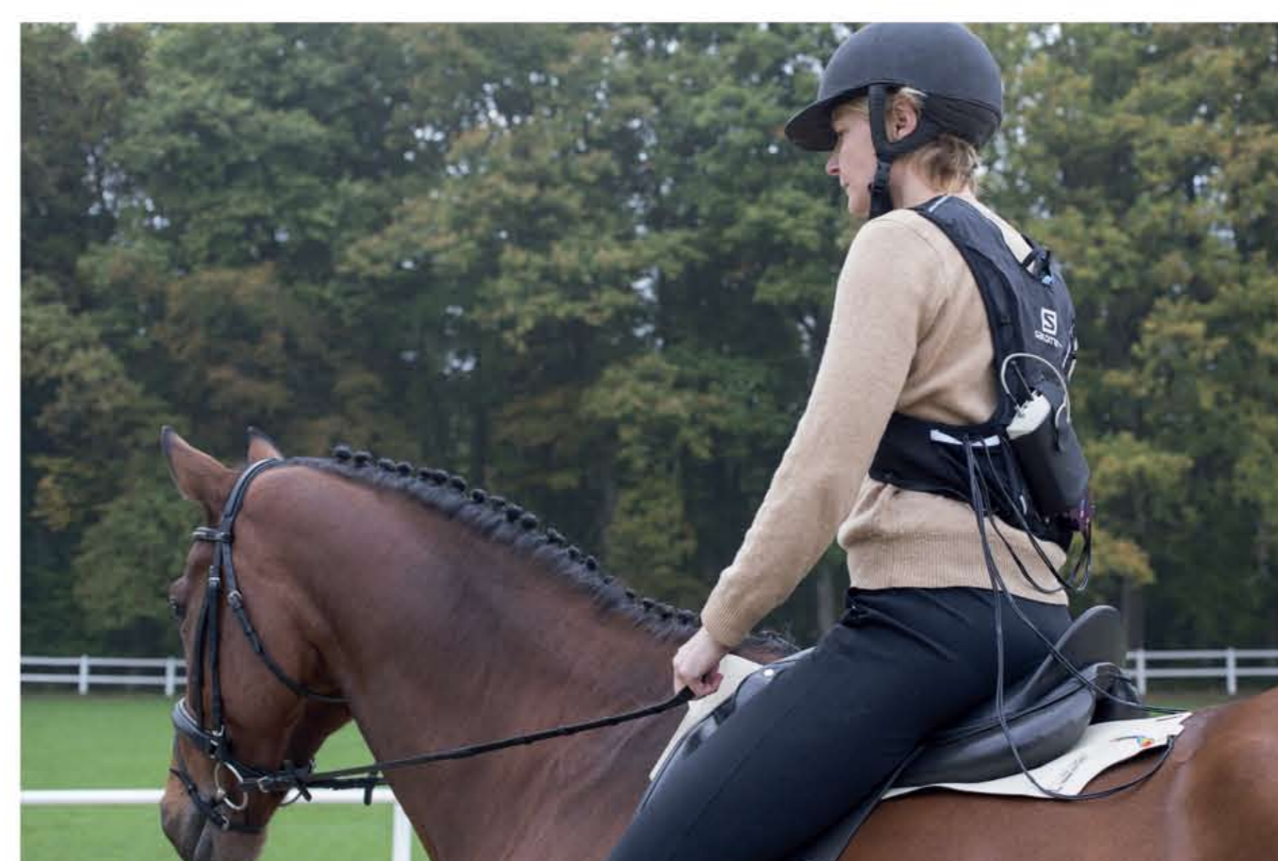
Fig.5: Horse-rider combination equipped with the saddle pressure measurement device.
